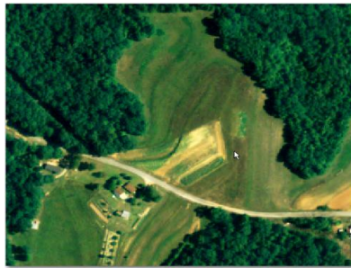
Figure 6. Produced from image and elevation data, orthophotos allow efficient image analysis of habitat, wetlands and vegetation/crops.
