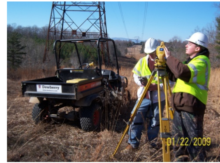
Figure 8. Field survey costs may be a hundred times more expensive, yet less valuable than aerial surveys from lidar or photogrammetry.
